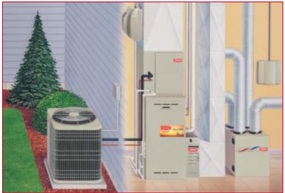
Central Air Conditioner and Gas Furnace System
